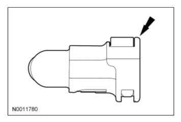
4. **NOTE:** If the retainer clip is properly installed, the tool should be locked into the quick connect coupling body and can only be removed when the center of the retaining clip is depressed.
