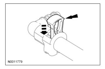
3. Push the retainer clip straight into the quick connect coupling body until it is flush with the top lip and the side of the connector body.
